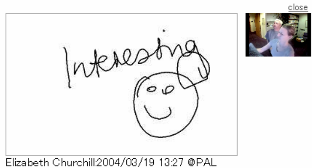
Figure 7 Enlarged scribble comment with video. When a user touches a thumbnail of scribble on the list, scribble image is enlarged and shown with video playing that captured when the user posted the scribble comment.
